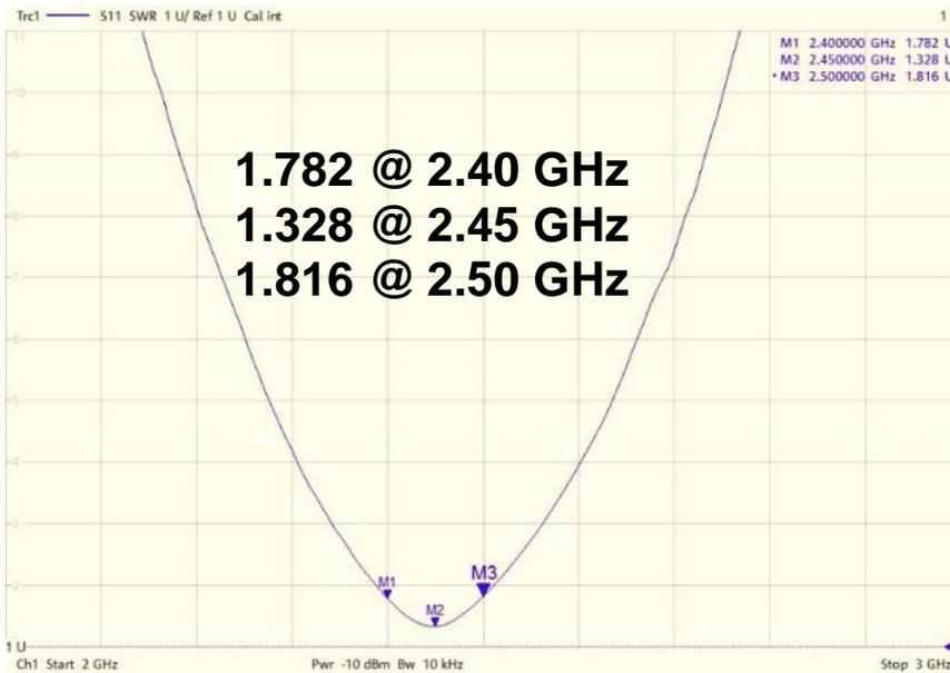
**Antenna on Type-2 Test Board ( Empty Space 6.3x4 mm &Thick ness 0.8mm)**
