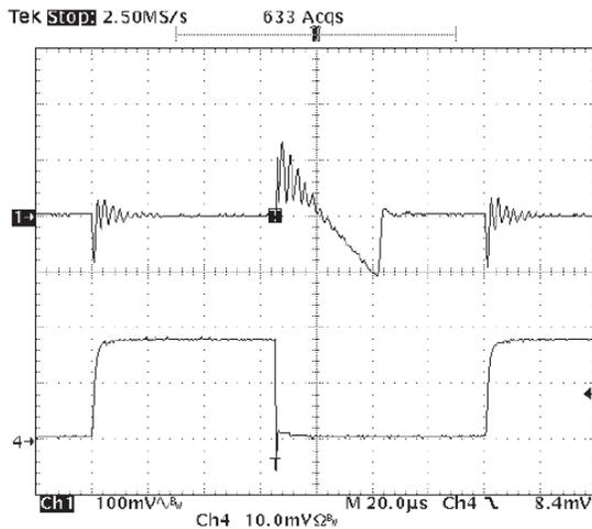
Fig. 16: Load Step Response 0mA to 800mA
