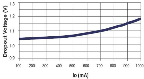
Fig. 5: Dropout Voltage vs Output Current
