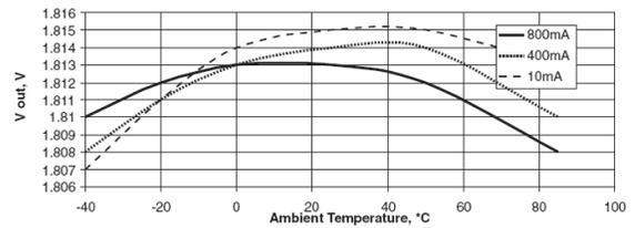
Fig. 14: Output Voltage vs Temperature
