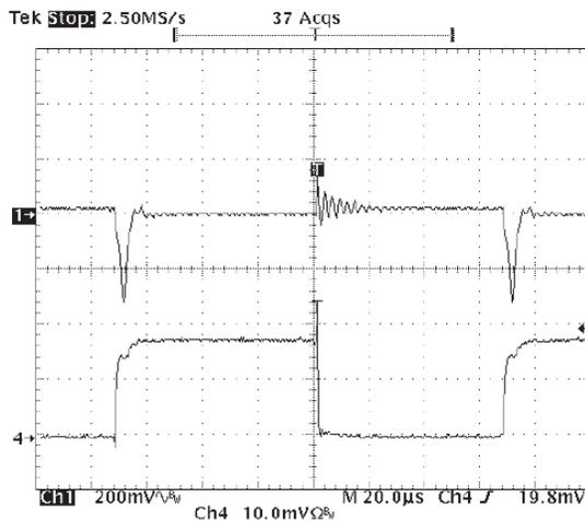
Fig. 17: Load Step Response 0mA to 800mA
