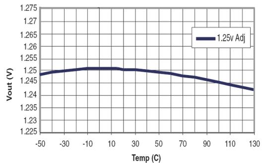
Fig. 8:  $V_{OUT}$  vs Temperature
