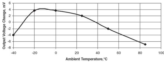
Fig. 13: Line Regulation vs Temperature
