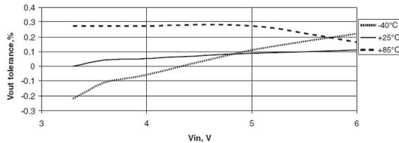
Fig. 15: Line Regulation over Temperature
