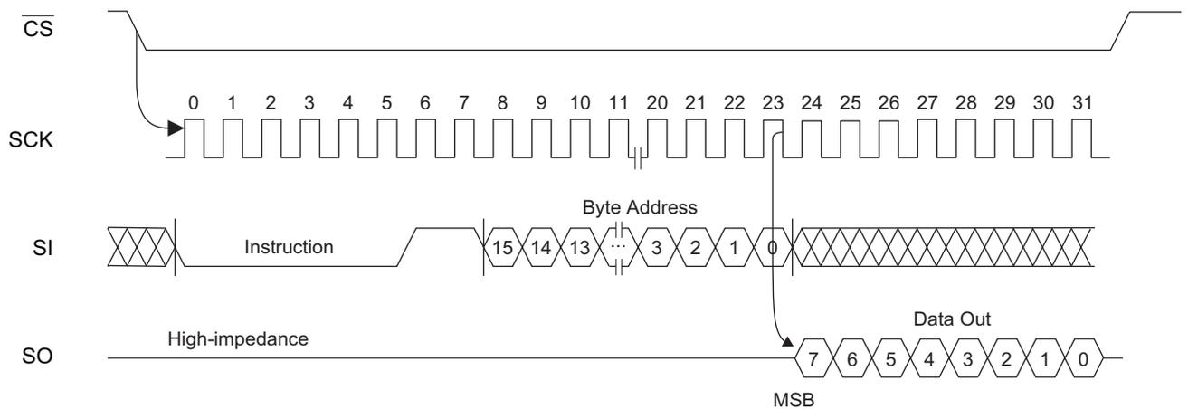
**Figure 7-7. Write Timing**
